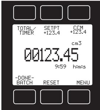
**Rollover** – The customer can also specify at the time of order what the totalizer is to do when the maximum count is reached. The following options may be specified:
