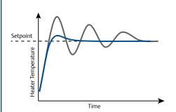
• PID feedback controller reduces overshoot and undershoot effects, resulting in steady heater temperature control
