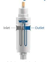
• Flow path design maximizes heat transfer to ensure complete sample vaporization
